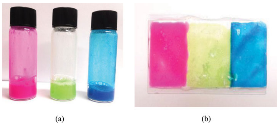
Figure 5. (a) Color LC capsules with red, green, and blue colors and (b) fabricated color PDLC device.
